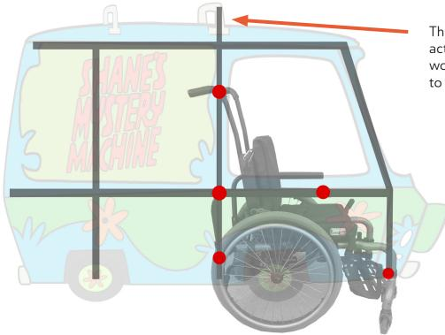
The van's rollbar on top would actually be the PVC frame and would serve as a parent handle to help push Shane if needed.
